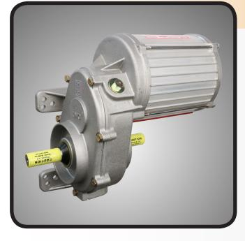
The Standard UMC® Power Saver® 4 center drive features an optimized helical gear design that offers longer life and quieter operation, cartridge output seals that eliminate shaft grooving and reduce oil leaks, and a single bolt junction box cover that makes installation and maintenance easier and faster. It is available with 7 output RPM options.
