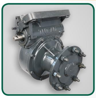
The UMC® TNT-U-AD™ gearbox is purpose built for higher performance and longer life. It features a 50:1 gear ratio, a 2.25" diameter output shaft, large input bearings, cartridge seals and enhanced gear material that allows for increased load capacity, reduced gear wear and lower operating temperatures. It is a direct replacement for its predecessor, the TNT-2-U™.
