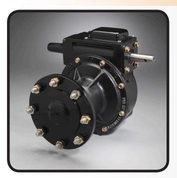
The UMC® 740-UV<sup>™</sup> gearbox features a 52:1 gear ratio, a 2.25" diameter extended output shaft, large input bearings, cartridge seals and enhanced gear material that allows for increased load capacity, reduced gear wear and lower operating temperatures.
